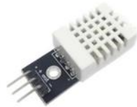
Fig 2.4 DHT22 Temperature and Humidity Sensor
